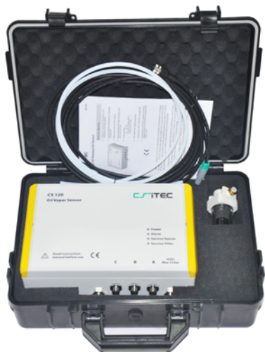
Portable CS 120-P with accessories connectable to CS 550
